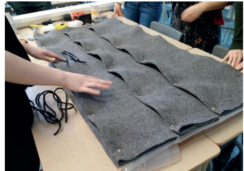
Assembly of pocket modules in recycled felt where the vegetable garden plants will be placed
