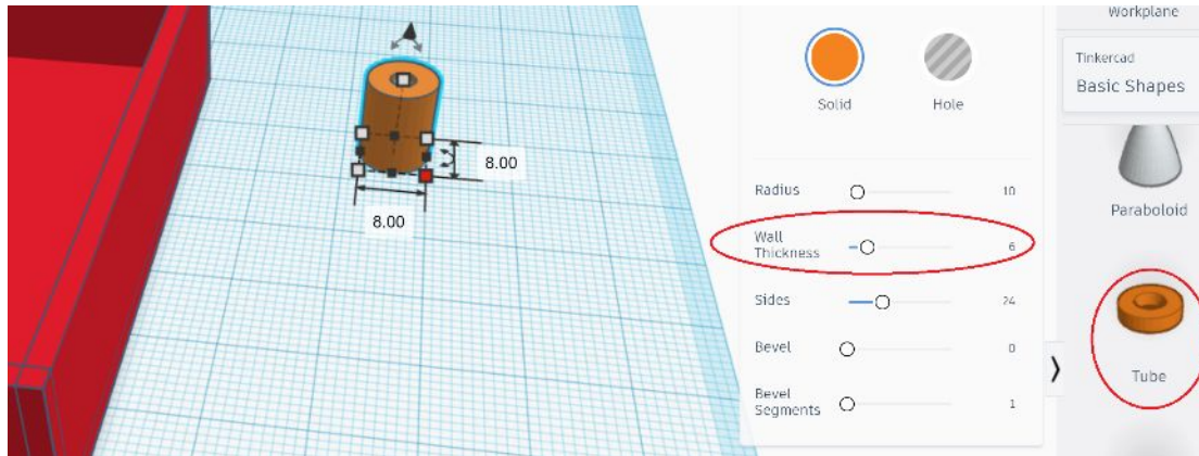
Making a tube with 2 mm inside diameter and 8 mm outside diameter
